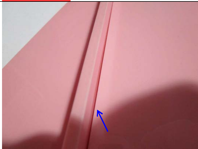
The tray panel is loosed (the glue is not firmly attached).
